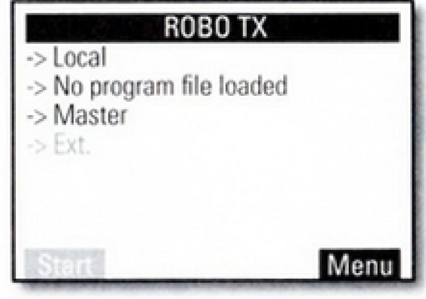
Master: The Controller, which is set as the master, receives control commands directly from the PC and passes these on to the extensions. Extension: The Controller, which is set as the extension, receives control commands only through the master.
