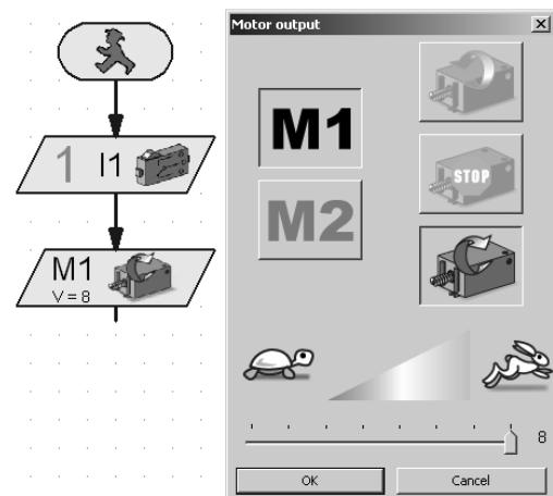
Here, you set the direction of rotation "clockwise" (green arrow). The connection M1 is already preset. Leave the slider control for the speed set on the far right. Then, the motor runs at full speed. Now, you can close the window with **OK**.
