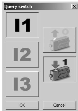
In this window, you can set which push-button switch (I1-I3) you want to query and if the switch is pressed (1) or not pressed (0). I1 and "switch pressed (1)" are already preset so that you can confirm with **OK**.
