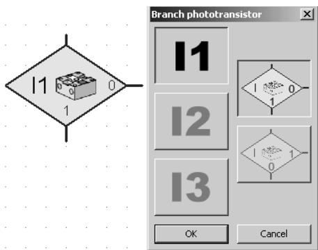
For querying of the phototransistor, you are to use the command "Branch phototransistor." Here, you have three connections as well. The program is set as follows: If the light barrier is interrupted (no light), go to the output 0. If the light barrier is not interrupted, go to the output 1.
