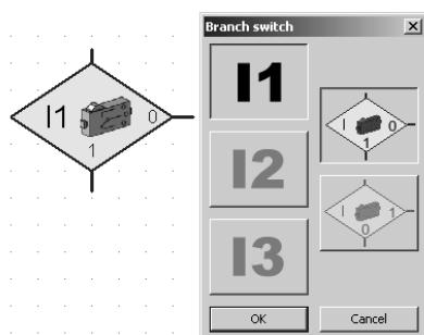
For querying of the switch, you are to use the command "Branch switch." Here, you have three connections. The program is set as follows: If the push-button switch is not pressed, go to output 0. If the push-button is pressed, go to output 1.
