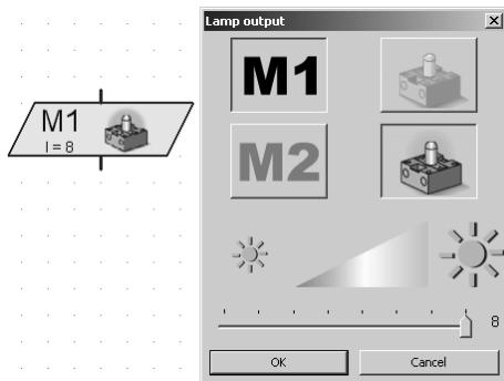
For the command "Lamp output," you also have the possibility of making various settings. You can set the brightness, the output (M1 or M2), and decide if the light is to be turned on or off.
