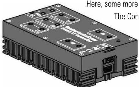
The Controller has three inputs (I1-I3) for connection of sensors, two outputs (M1-M2) for the connection of actuators, a DC jack socket for the connection of a power supply unit (9V), two connecting sockets for a 9V battery tray or rechargeable battery pack, a mini-USB connection for data transmission from the PC to the Controller and a LED as an equipment-on indicator light.
