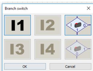
To query the push-button switch, use the command "Branch switch". Here, you have three connections. The program is set as follows: If the push-button switch is not pressed, go to output 0. If the push-button is pressed, go to output 1.
