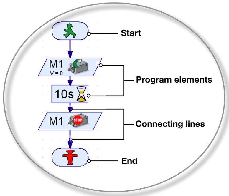
When the program is started, the routines are run one after the other. A control program in ROBO Pro Light begins with a little green traffic light figure (Start element) and ends with a little red traffic light figure.
