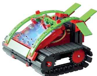
■ Now that you have already tested how a tracked vehicle moves forwards and backwards, as well as changing direction, this is a new challenge for you. Modify your vehicle so that it can recognize and automatically drive around obstacles with the aid of two push-button switches on the front.
