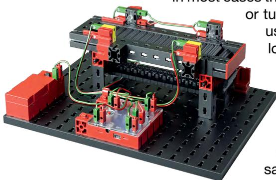
The conveyor belt consists primarily of a supporting construction. It supports the chain bearings (sprockets), the drive chain and the chain attachments as well as the drive station (drive sprocket, bearing, gearbox, motor) and various safety devices. Build the model using the assembly instructions and connect the cables according to the circuit diagram.
