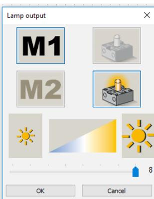
For the command "Lamp output," you also have the possibility of making various settings. You can set the brightness, the output (M1 or M2), and decide if the light is to be turned on or off.
