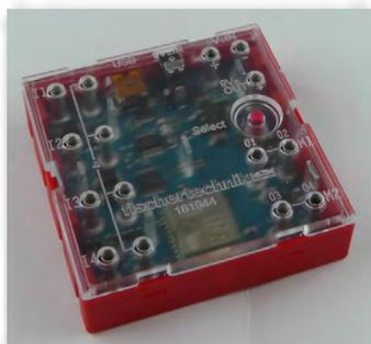
■ The BT Smart Controller is the heart of this ROBOTICS construction set. Although you cannot see them, the Controller module has a number of electronic components. The interplay of these components with your computer and a control program allows you to control the models in the ROBOTICS BT Smart Beginner Set.
