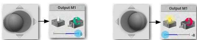
At the conclusion, press the push-button switch. The depiction of I1 in the “Inputs” window changes from “0” to “1”. The red direction arrow also changes.
