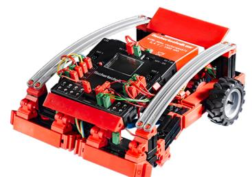
Then you can get started with the programming. The lawn is symbolized by the white area of our soccer stadium course 1b, which is bordered by a black edge. The lawn mower is not to pass over this edge, because otherwise, for example, it will end up on the synthetic running track. If an obstacle appears on the lawn, the robot is to avoid it when it runs into it. In addition, the cutter bar is to be turned off when an obstacle is detected.
