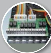
**Port:** PCB with relays to reverse polarity of motor, multi pin connector (26 pins, grid 2,54mm) and in addition PCB terminals with push in connection for all I/O
